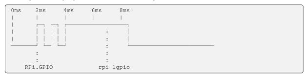
RPi.GPIO reports the edge at 2ms, then suppresses the edges at 3ms and 4ms because they are within 3ms of the last edge. By contrast, rpi-lgpio ignores the first and second rising edges (because they didn't stay stable for 3ms) and only reports the third edge at 7ms (after it's spent 3ms stable).
