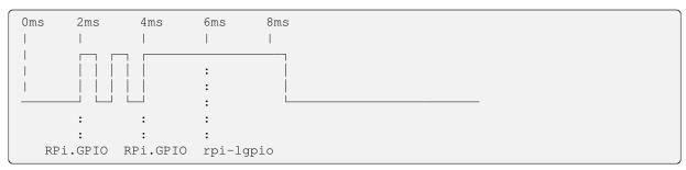
In this case, RPi.GPIO reports the switch *twice* because the third edge is still 2ms after the first edge. However, rpilgpio only reports the switch *once* because only one edge stayed stable for 2ms. Also note in this case, that rpi-lgpio's report time has moved back to 6ms because it's not waiting as long for stability.
